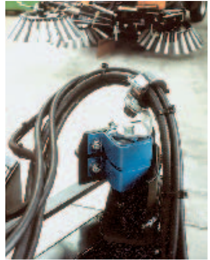
Suspension of a brush in road sweeper
