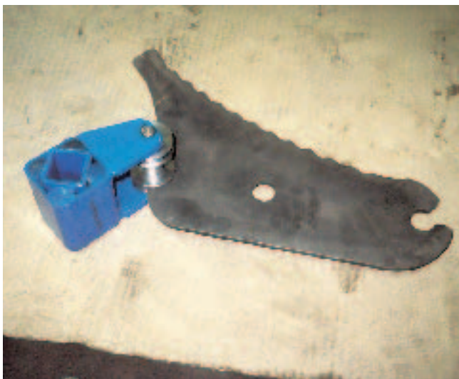
Elastic suspension of shaping knife in baler
